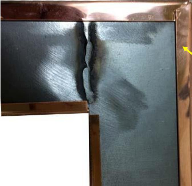
**Pictured** is the top corner section of a frame from the back to show this wrapping technique
